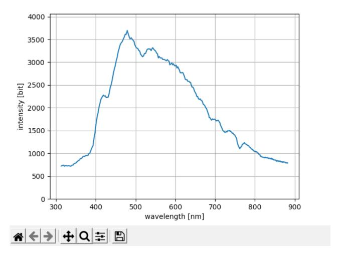
Now, you can decide whether to save the spectrum into a file, add it to an average spectrum, or use it in an absorption calculation.
