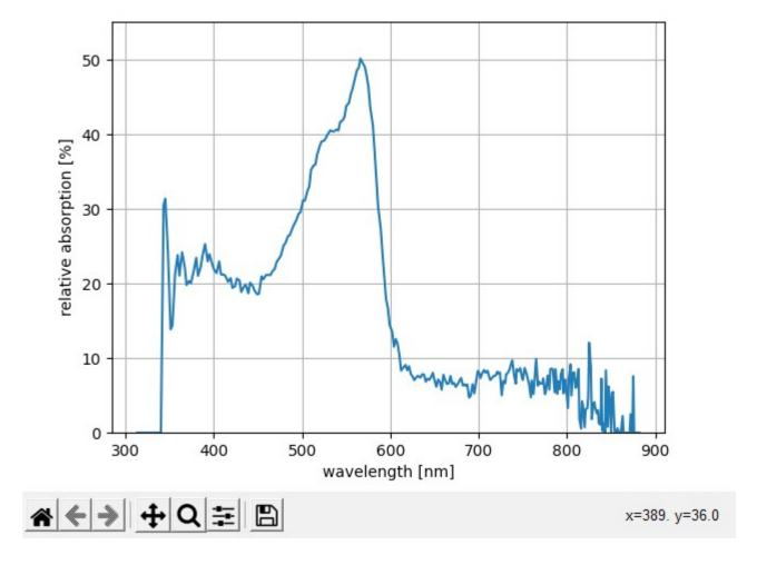
You can save the absorption spectrum by pressing the *SAVE ABS* button. To load a saved absorption spectrum, navigate to the *MEAS* page and press the *LOAD* button.
