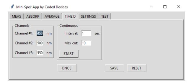
Time D is the page for making measurements in the time domain, specifically generating time series data for selected wavelengths.
