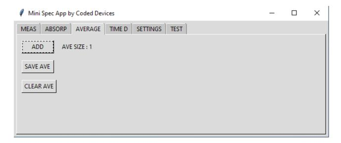
Use several measured spectrums to create an average spectrum. This is a simple method to attenuate noise and other irregularities found in measured signals. It is effective as long as the measuring conditions stay unchanged.
