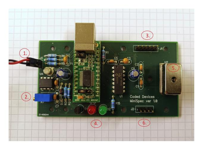
Note! The instrument is designed to be used with a plastic enclosure. The electrical connections are accessible from the bottom and a short circuit may occur if the instrument is placed on conductive material or parts. If your application requires using the device without the enclosure, ensure there is no risk of short circuits by using insulating pads underneath.
