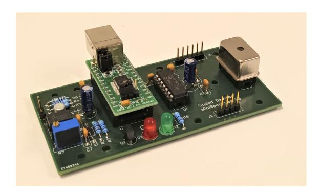
The Mini Spectrometer is a compact spectrometer operating in the visible part of the spectrum. It is based on Hamamatsu Photonics C12880MA spectrometer head.
